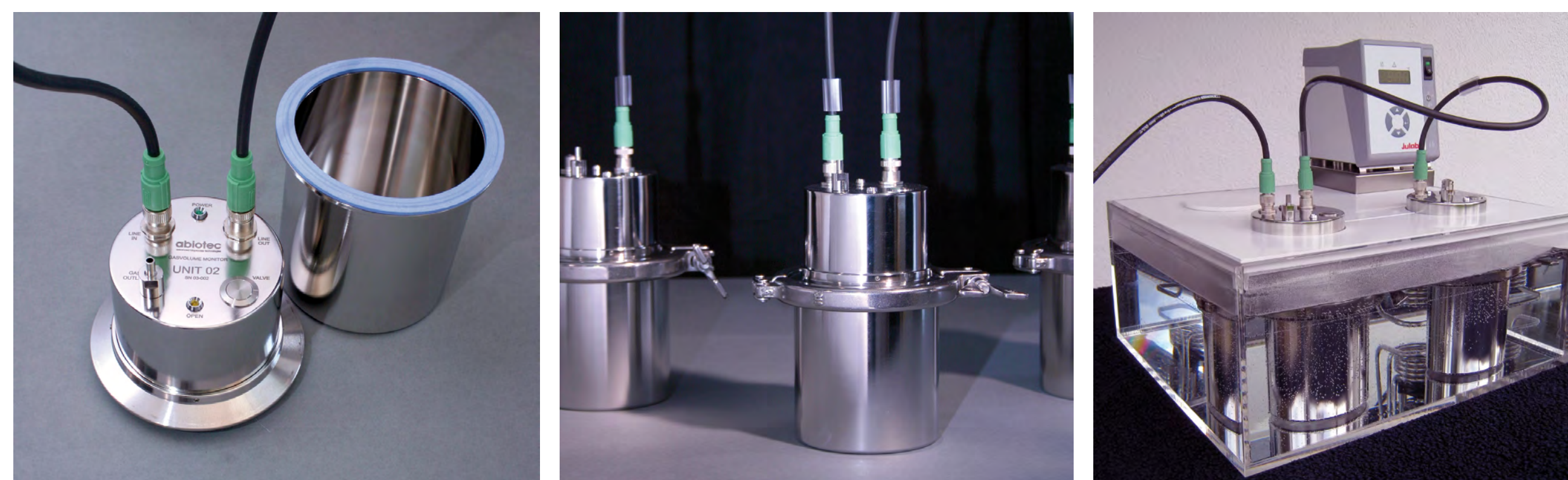
Fig. 1: Determination of gas formation activity by means of the Gas Volume Monitor from abiotec AG.
